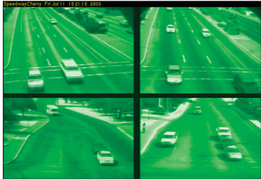
Video cameras at signalized intersections are used to collect data on traffic queues and delays. Cameras on the four approaches to Speedway and Cherry are shown in the above photo.
