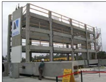
The experimental program culminated with a large demonstration test at the NEES@UCSD Large High Performance Shake Table at Englekirk Structural Engineering Center, the largest shake table in the U.S. The test specimen was a three-story precast concrete structure at half-scale designed with the emerging methodology. The one-million pound structure had the largest footprint of any structure ever tested on a shake table in the U.S.
