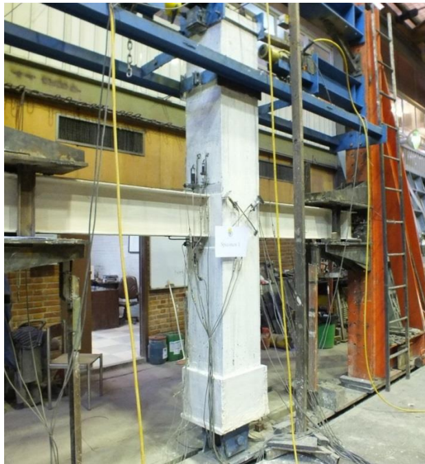
Figure 1: Testing a RCS connection [13].
