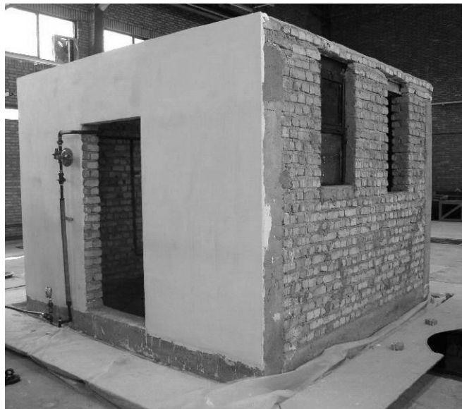
Figure 3: Testing a confined masonry structure on the shaking table of Sharif University [20].
